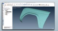
**MEASURE** - Scan and capture measurement data with the peel 2 3D scanner and 'One-Button' export the point cloud data to Verisurf.
