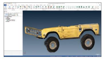
Peel 2 features 'one-button' export of high-quality point cloud data directly into Verisurf software for measurement processing. From there Verisurf is able to measure, mesh, model, inspect and report as needed, establishing and maintaining a digital thread forward.
