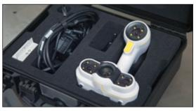
The peel 2 3D scanner comes with everything you need to be productive, right out of the box, including the scanner, a calibration plate, positioning targets, a power supply, and a USB stick containing the manual and scanner software installer. Add to this your choice of Verisurf application suite and you have the power to finish the job.
