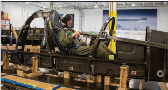
*Chief test pilot, Bill Shoemaker, conducts ergonomic test in the carbon fiber, XB-1 nose bay sub assembly.*
