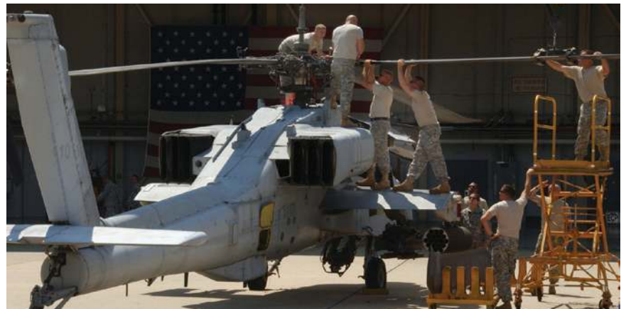
U.S. Soldiers from the Army National Guard replace rotor blades on Apache.
