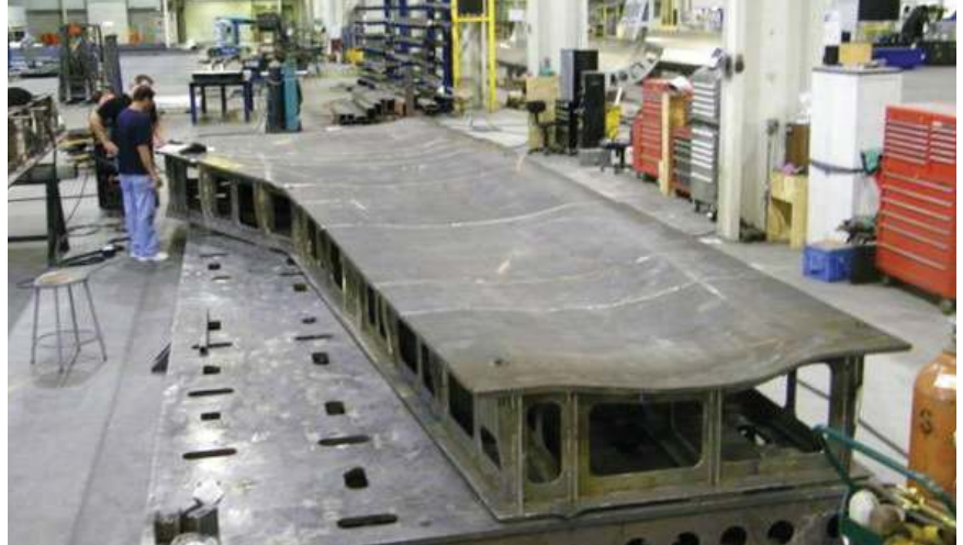
A large Invar bond tool used for wing lay up.
