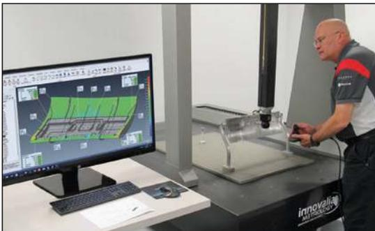
*Finished wing part is inspected against the nominal 3D CAD design using Verisurf Software, running a Spark Gage programmable CMM. Verisurf can interface with this otherwise closed CMM device through Verisurf Universal CMM Software. The software allows Verisurf to drive measuring hardware devices that do not comply with the I++ open protocol. This applies to both new and legacy CMMs, regardless of controllers or outdated software.*
