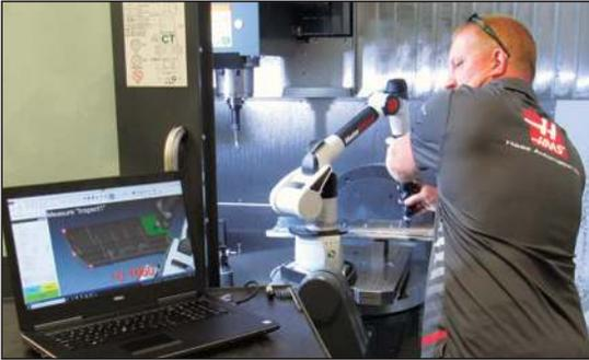
*Haas F1 Team inspects 100% of all parts produced. Inspecting parts in process using a Master3DGage, portable CMM saves time by eliminating the need to re-fixturing parts or move them around the shop.*
