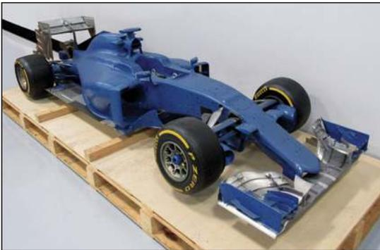
*Haas F1 Team wind tunnel model produced at 60% of scale emphasizes the importance of precision as any deviation from nominal will be amplified at full scale.*
