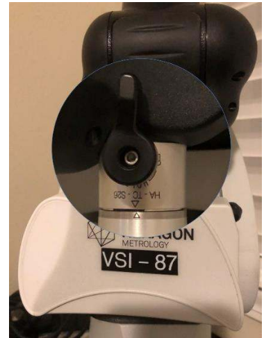
Above – Scanner attached and locked, note the Alignment symbols ( \nabla \Delta ) on the Scanner and Connector.
