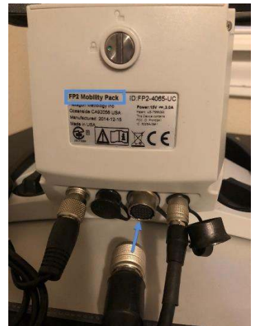
Above – Scanner attached and locked, note the Alignment symbols ( \nabla \Delta ) on the Scanner and Connector.
