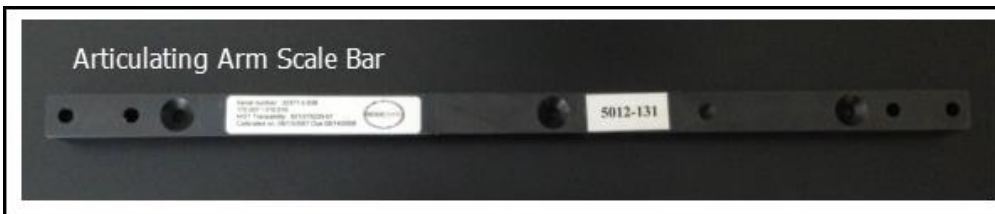
Above: Laser Tracker Scale Bar with Three Certified Distances.
