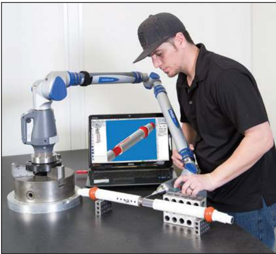
The data was captured to Verisurf Reverse™ using a Faro portable CMM with a contact probe, which was the right choice given the centricity of part.
