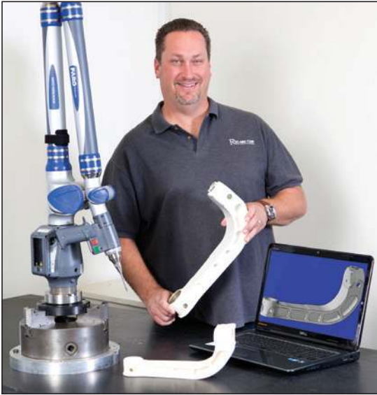
Jason Collins, General Manager of Roc-Aire holds redesigned and manufactured main gear strut; 3D printed engineering prototype, produced at 2:3 scale (foreground). 3D prototype used for engineering review and design approval.
