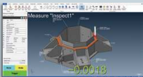
Inspect Part to CAD Datums
